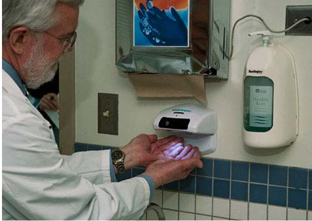
The HyGreen hand-hygiene sensing device detects the alcohol in the gel that James L. Cook, MD, uses to wash his hands and sends an infrared signal to his badge to record the washing event. If he enters a 7-foot zone near a patient's monitor without washing his hands, the badge will vibrate as a reminder. [Photo by Ted Grudzinski / AMA]
